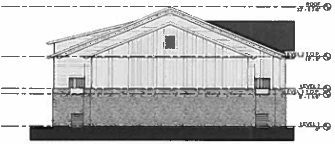
② BUILDING C - WEST ELEVATION 1/8" = 1'-0" NO. OF WINDOWS 1 000 NO. OF DOORS 2 000 NO. OF BALCONIES 0 000 NO. OF STAIRS 1 000
