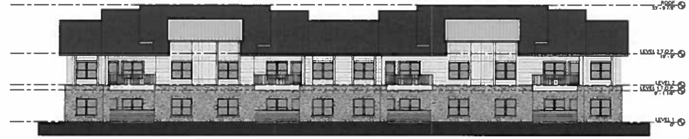
① BUILDING C - NORTH ELEVATION 1/8" = 1'-0" NO. OF WINDOWS 11 000 NO. OF DOORS 2 000 NO. OF BALCONIES 2 000 NO. OF STAIRS 1 000
