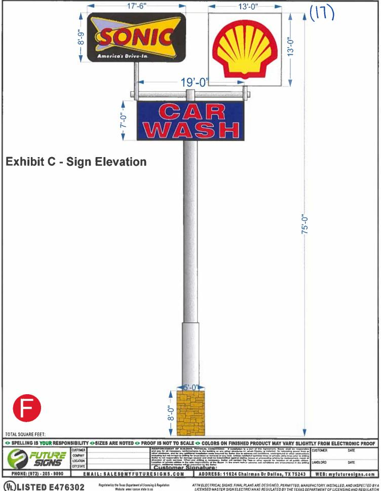
ATTN ELECTRICAL SIGNS: FINAL PLANS ARE DESIGNED, PERMITTED, MANUFACTORY, INSTALLED, AND INSPECTED BY A LICENSED MASTER SIGN ELECTRICIAN AS REGULATED BY THE TEXAS DEPARTMENT OF LICENSING AND REGULATION
