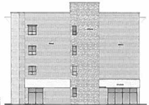
END ELEVATION - BUILDINGS 2,3,4 1/8" = 1'-0"
