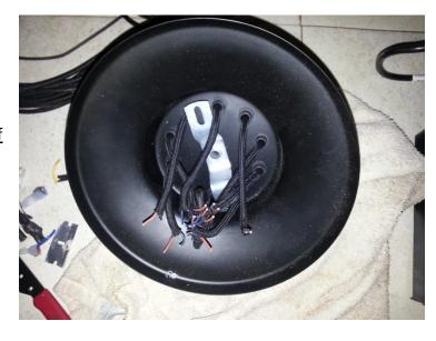
Below is a custom 10 wire. We cut the wires to be <u>50" long AFTER assembling the bulbs and dry fitting the entire light.</u> This gave us a 10 wire chandelier, 48" in diameter, with a 12" wire drop, and a 10" bulb drop as shown below.
