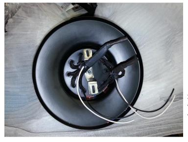
On each side – bundle/separate the blue wires with dark wire, and red wires with light wire. Snip the wires so they are equal length so they are easier to connect.
