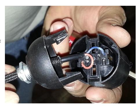
Step 6: The base is assembled last – as this is where you can shorten the wires if needed.
